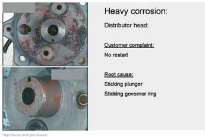
Figure DF-36: Example of Corrosion in Field Pump Caused by Free Water in Diesel Fuel
