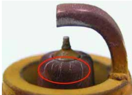
Figure G-19: Catalyst Thermal Damage by Misfiring of Spark Plugs Coated in Iron (UAE market, mileage 50,000km)
