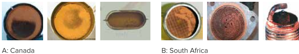
Figure G-15: Evidence of MMT's Impact on Canadian and South African Vehicles
